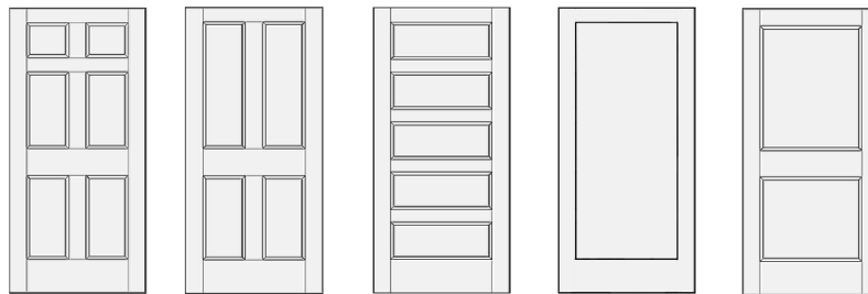
F9130 1-7/16 Fire Rated Raised Panel Ovolo Sticking F9244 F9255 F9220 3/4 Fire Rated Flat Panel Ovolo Sticking F9282
